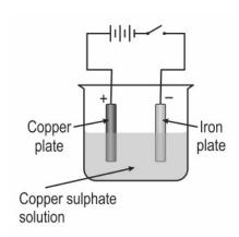
Q:  $\frac{1}{2}$  After a few minutes, even before he turned the switch on, he noticed that copper was deposited on the iron plate.
